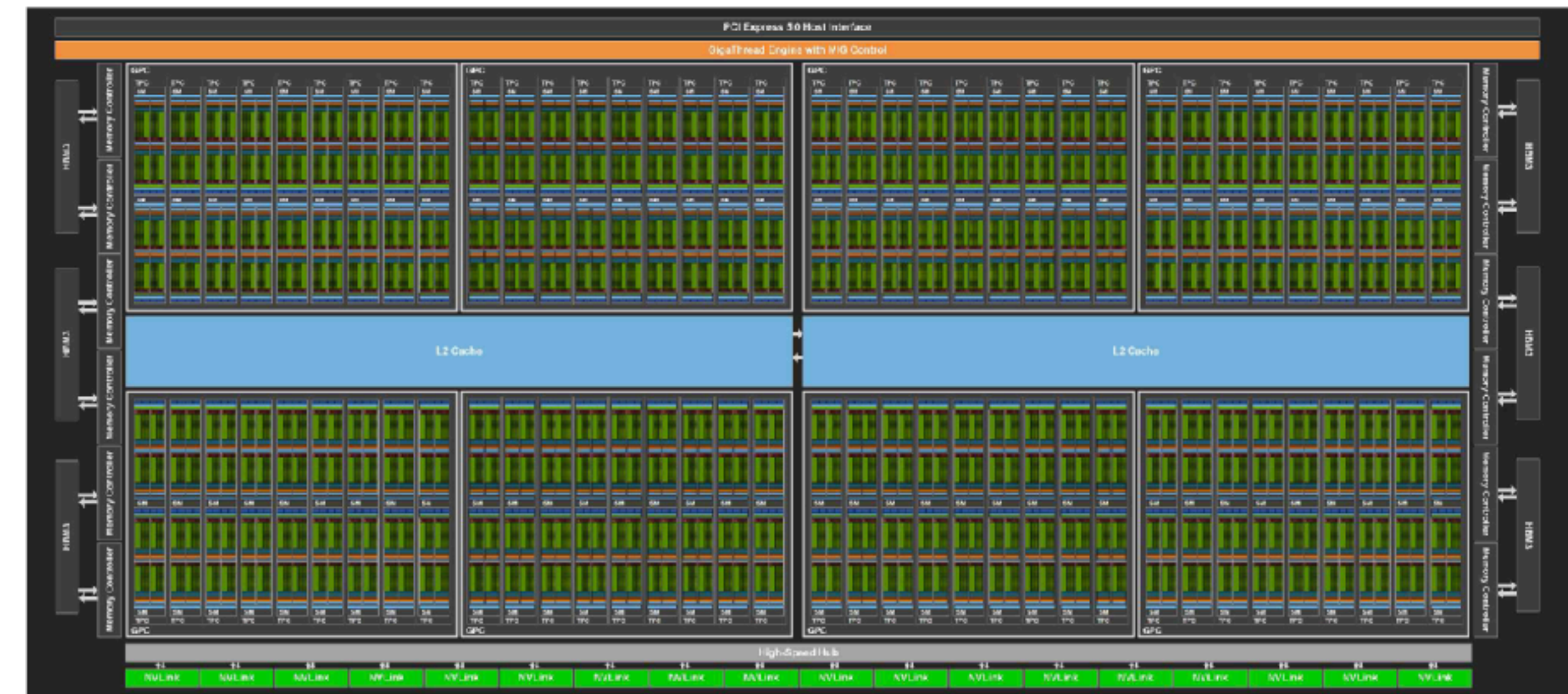
GH100 Full GPU with 144 SMs [1]
