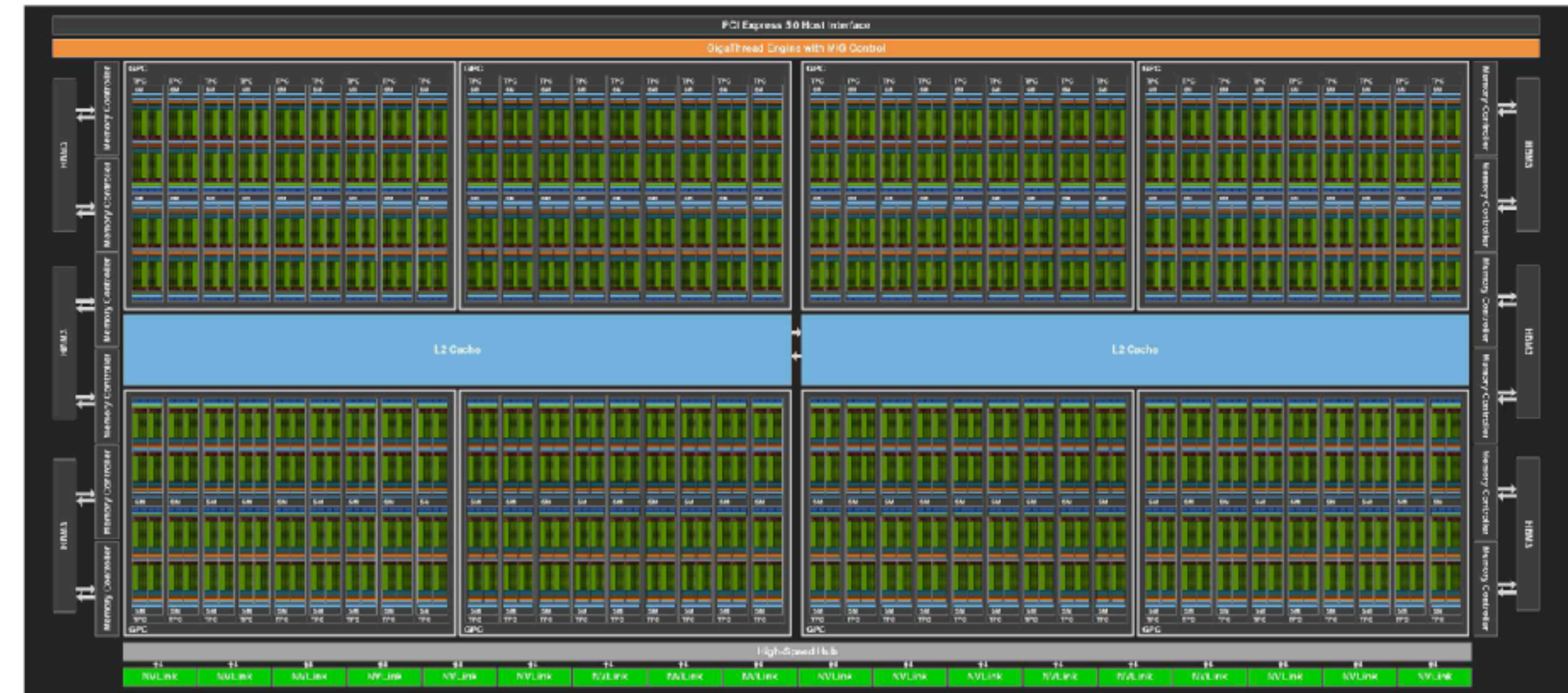
GH100 Full GPU with 144 SMs [1]
